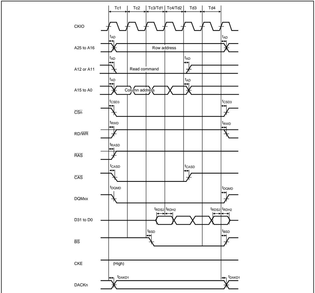
**Figure 24.31 Synchronous DRAM Burst Read Bus Cycle
