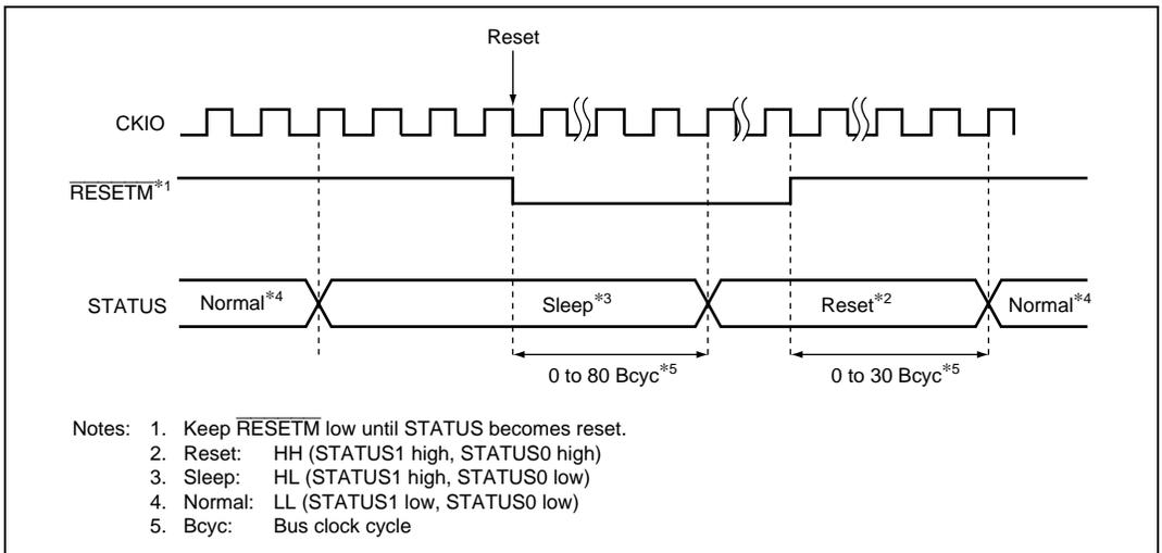
Figure 22.9 Sleep to Manual Reset STATUS Output
