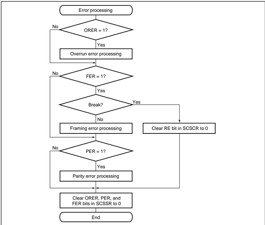
**Figure 14.10 Sample Flowchart for Receiving Serial Data (cont)**
