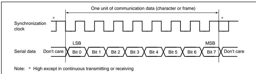
**Figure 14.17 Data Format in Clock Synchronous Communication**
