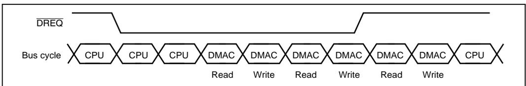
**Figure 9.15 DMA Transfer Example in the Burst Mode**
