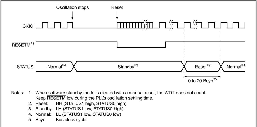
Figure 22.6 Software Standby to Manual Reset STATUS Output
