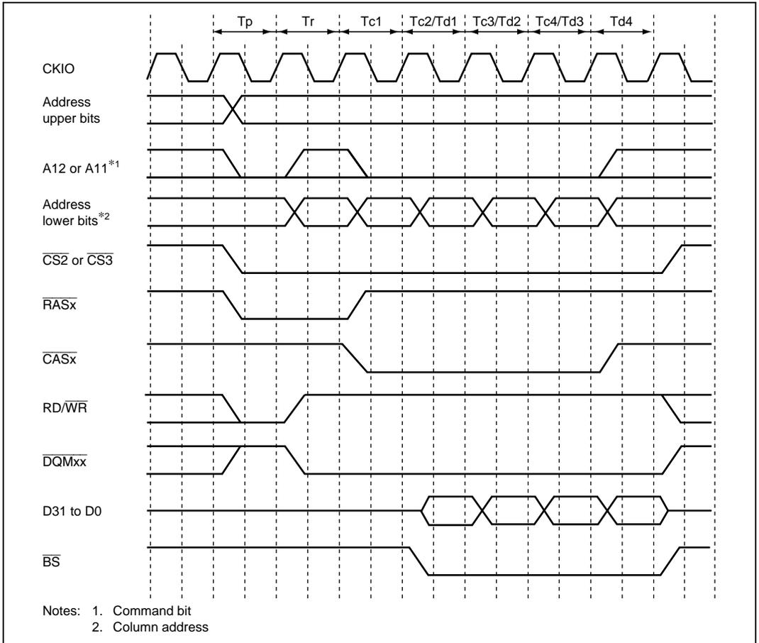
**Figure 8.20 Burst Read Timing (Different Row Addresses)**
