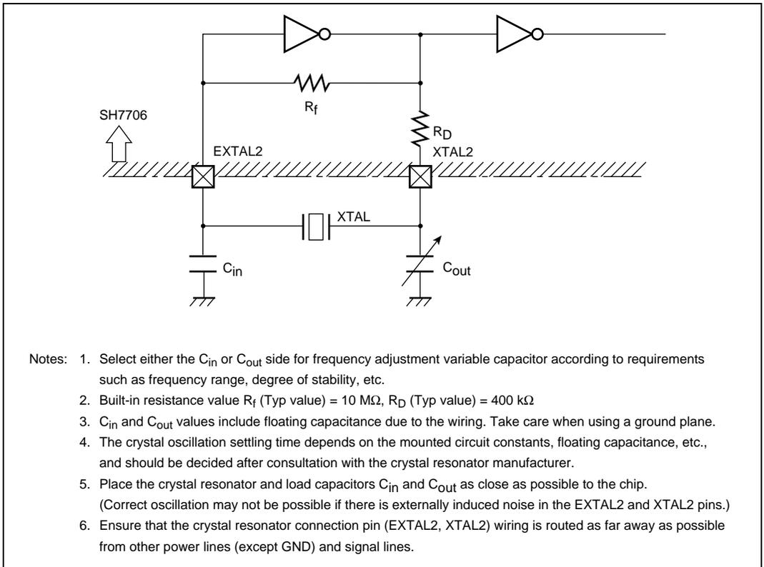
**Figure 13.5 Example of Crystal Oscillator Circuit Connection**
