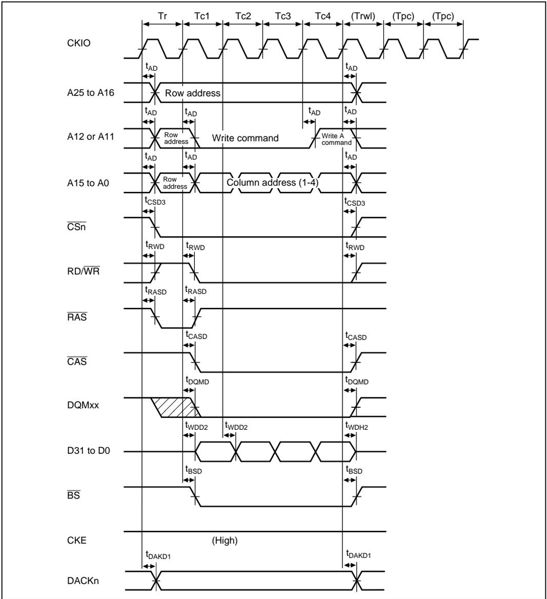
**Figure 24.28 Synchronous DRAM Write Bus Cycle**
