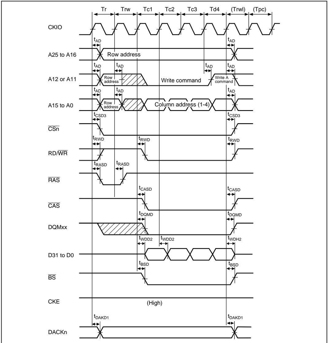
**Figure 24.29 Synchronous DRAM Write Bus Cycle**
