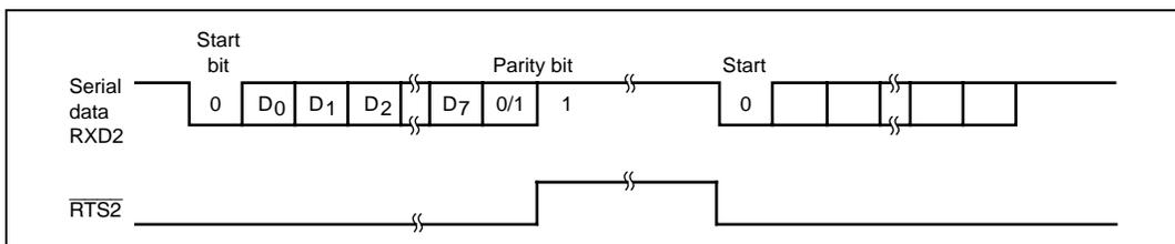
**Figure 16.12 Example of Operation Using Modem Control ( $\overline{\text{RTS2}}$ )**
