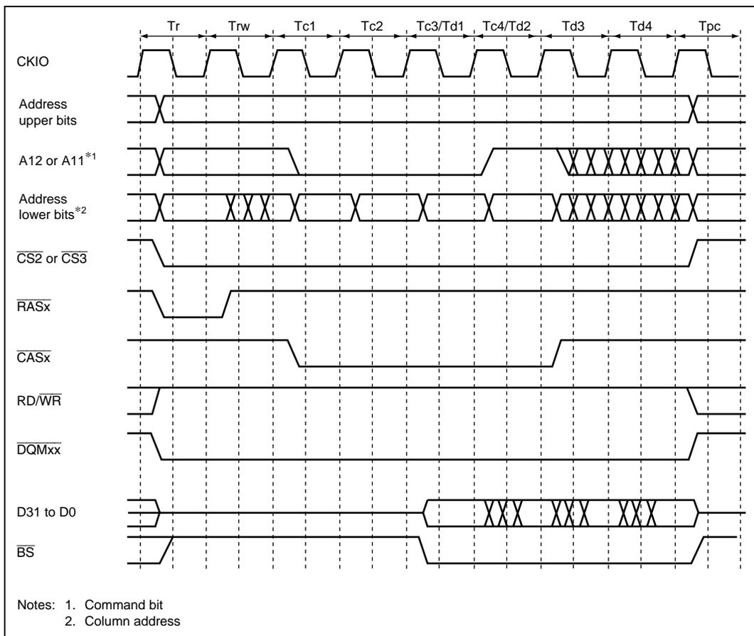
**Figure 8.14 Synchronous DRAM Burst Read Wait Specification Timing**
