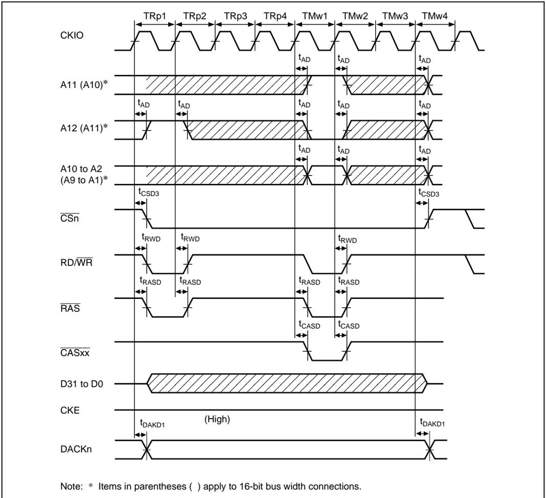
**Figure 24.39 Synchronous DRAM Mode Register Write Cycle**
