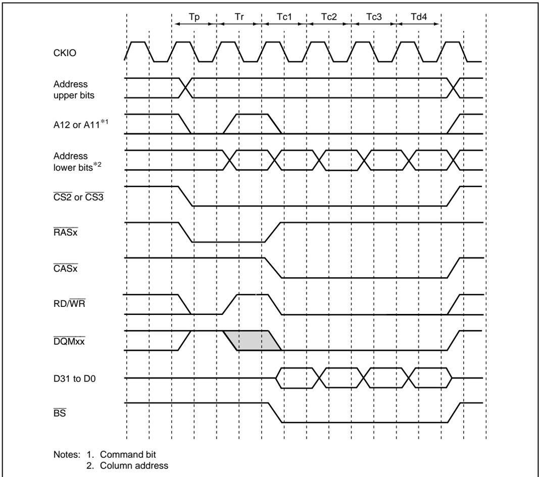
**Figure 8.23 Burst Write Timing (Different Row Addresses)**
