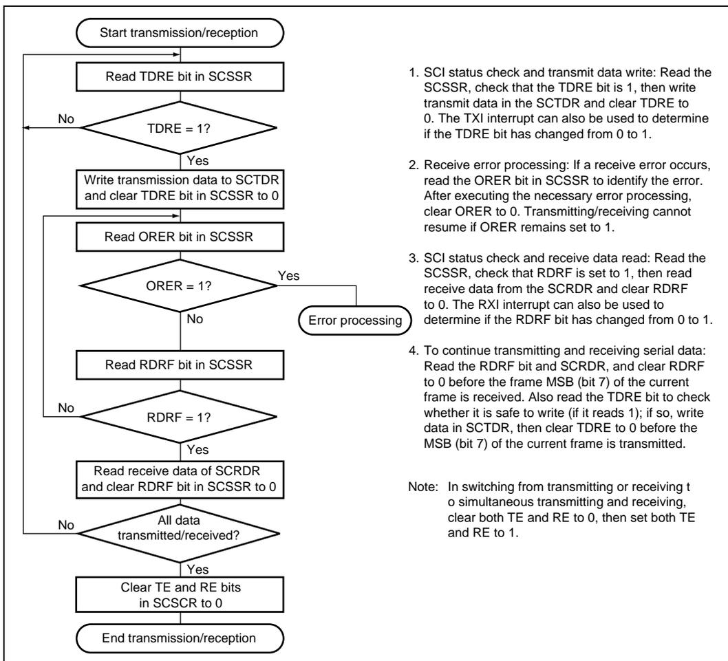
**Figure 14.23 Sample Flowchart for Serial Data Transmitting/Receiving**
