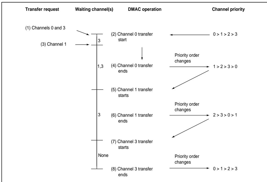
**Figure 9.4 Changes in Channel Priority in Round-Robin Mode**
