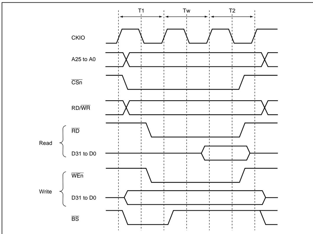
**Figure 8.9 Basic Interface Wait Timing (Software Wait Only)**
