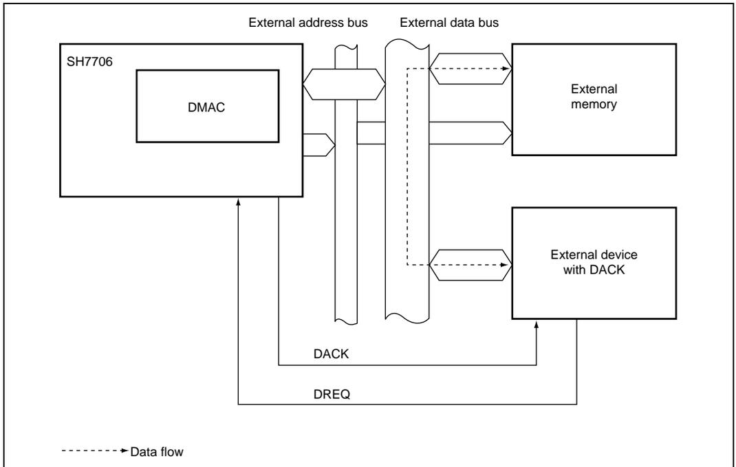
**Figure 9.11 Data Flow in the Single Address Mode**
