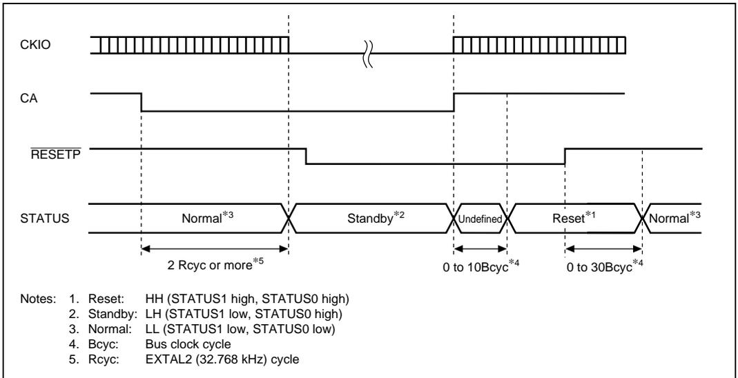
**Figure 22.10 Hardware Standby Mode
