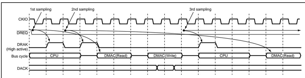
**Figure 9.18 Cycle-Steal Mode, Level Input (CPU Access: 3 Cycles)**
