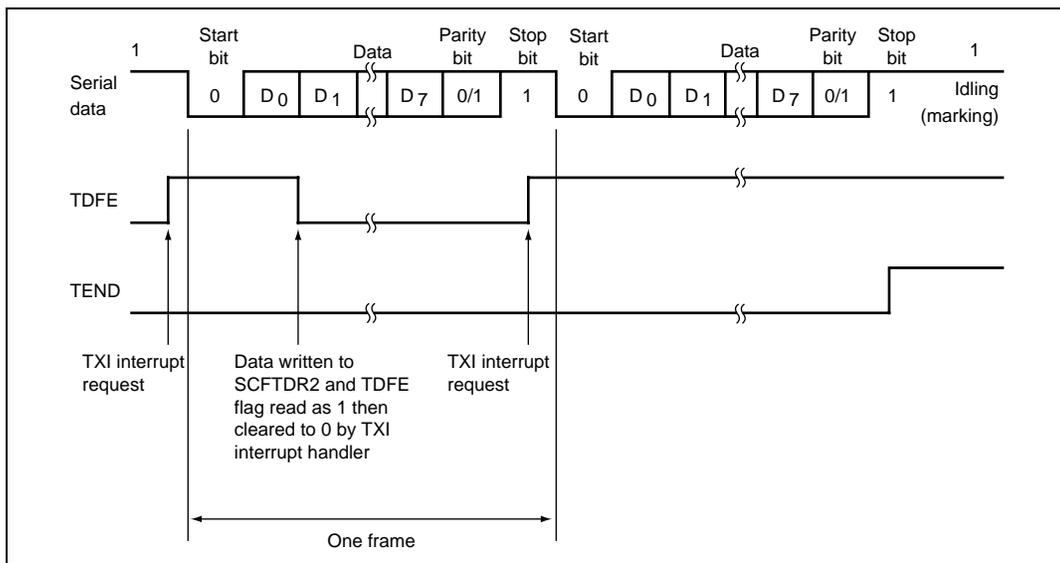
**Figure 16.7 Example of Transmit Operation
