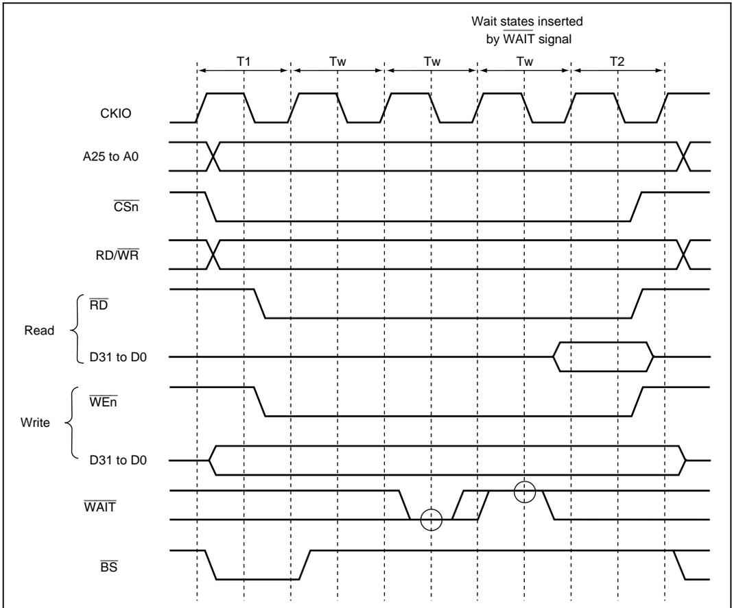
**Figure 8.10 Basic Interface Wait State Timing**
