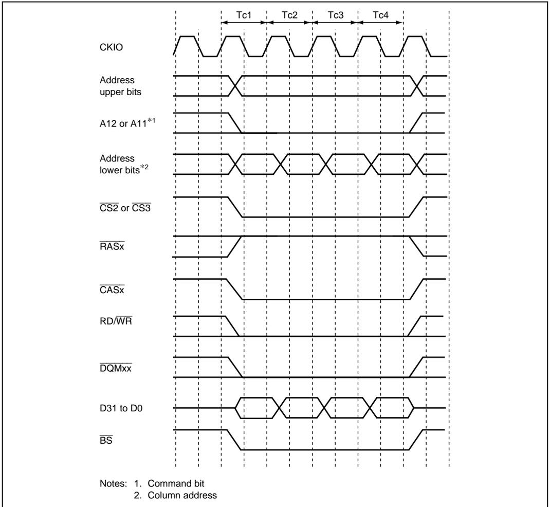
**Figure 8.22 Burst Write Timing (Same Row Address)**
