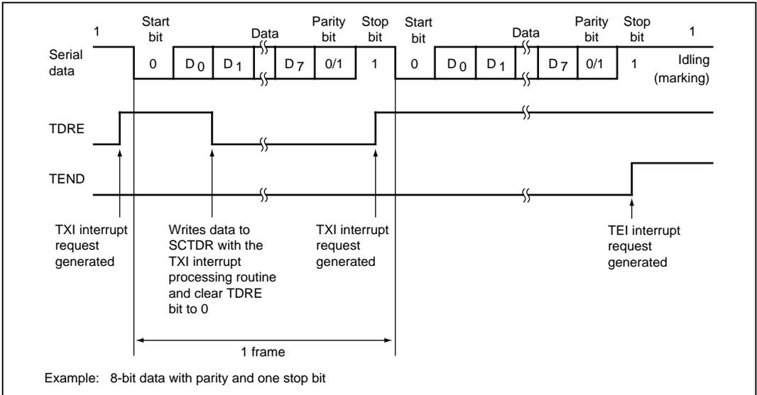
**Figure 14.9 SCI Transmit Operation in Asynchronous Mode**
