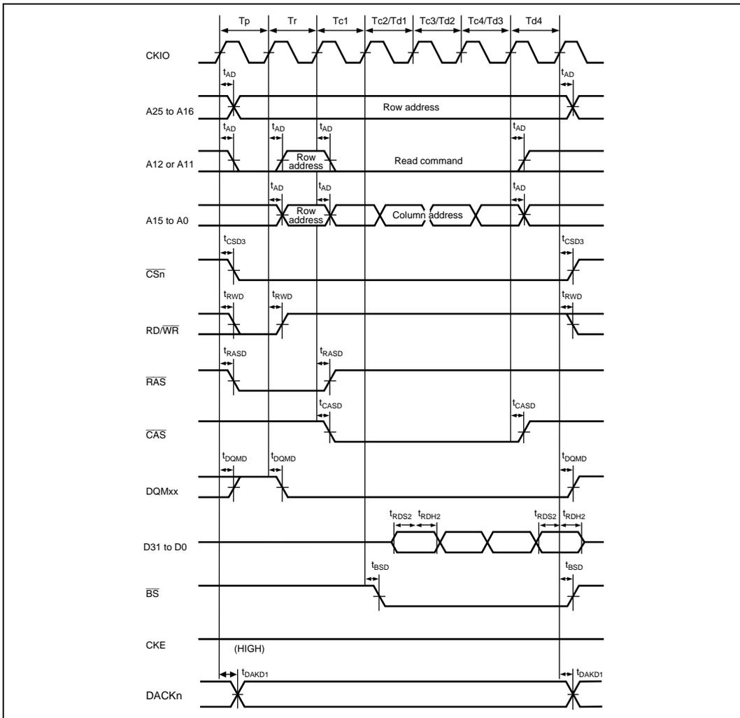
**Figure 24.32 Synchronous DRAM Burst Read Bus Cycle**
