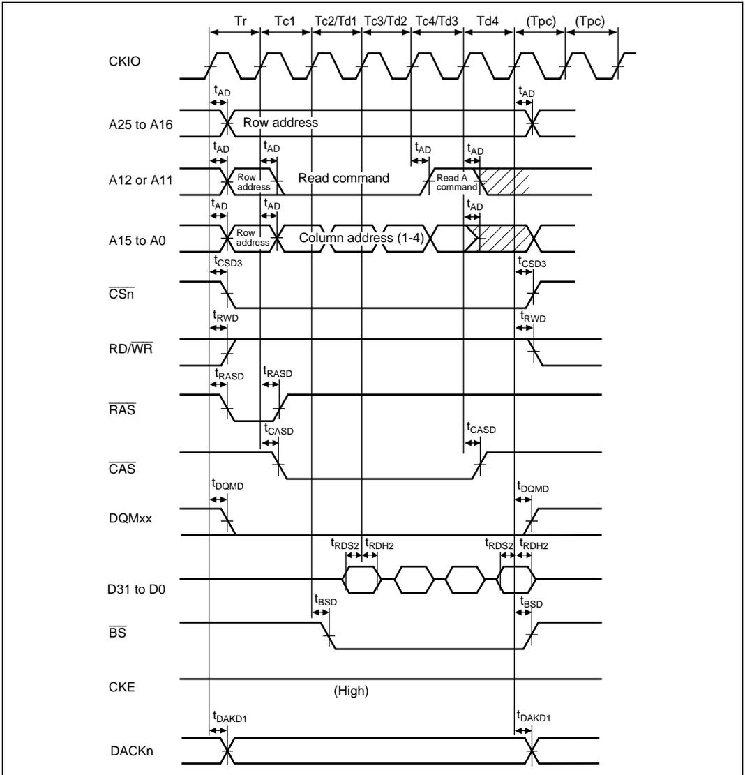
**Figure 24.24 Synchronous DRAM Read Bus Cycle**
