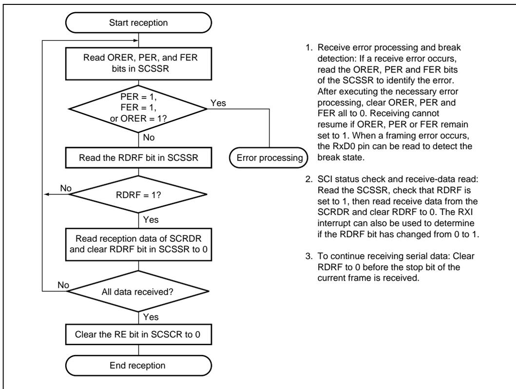
**Figure 14.10 Sample Flowchart for Receiving Serial Data**
