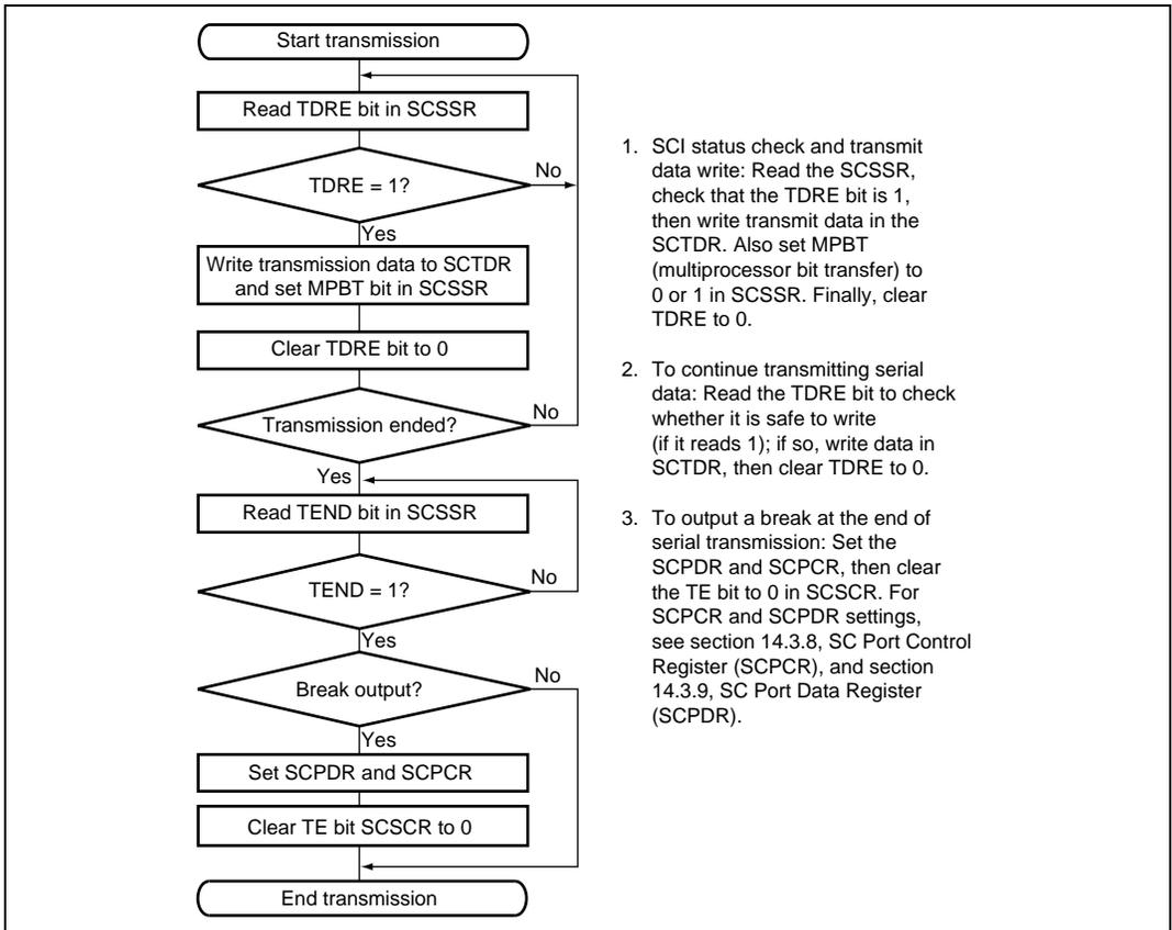
**Figure 14.13 Sample Flowchart for Transmitting Multiprocessor Serial Data**
