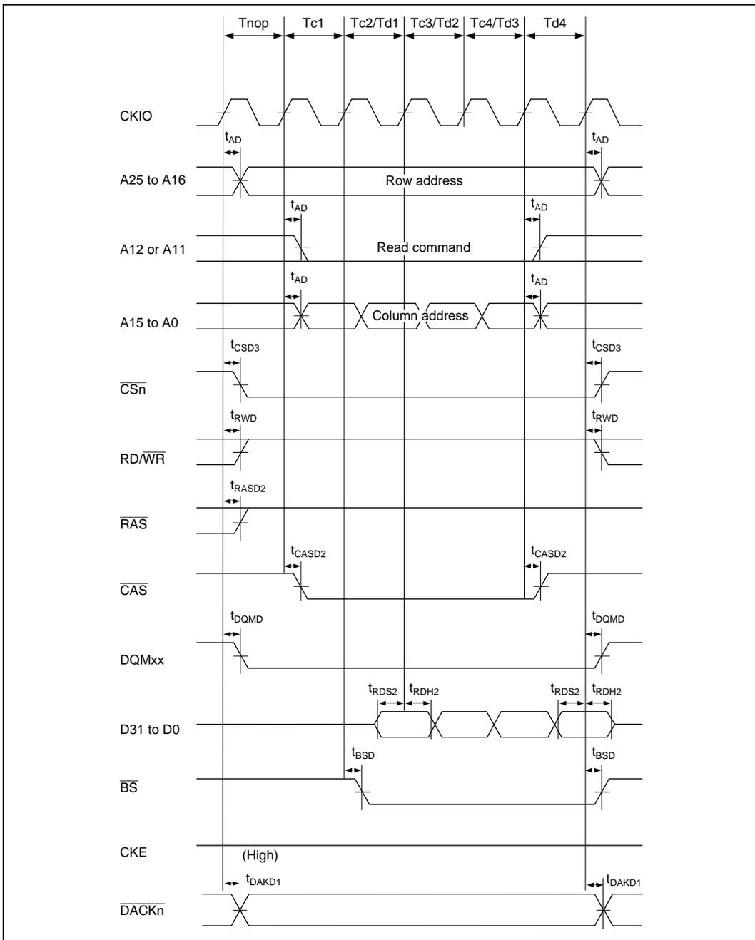
**Figure 24.30 Synchronous DRAM Burst Read Bus Cycle
