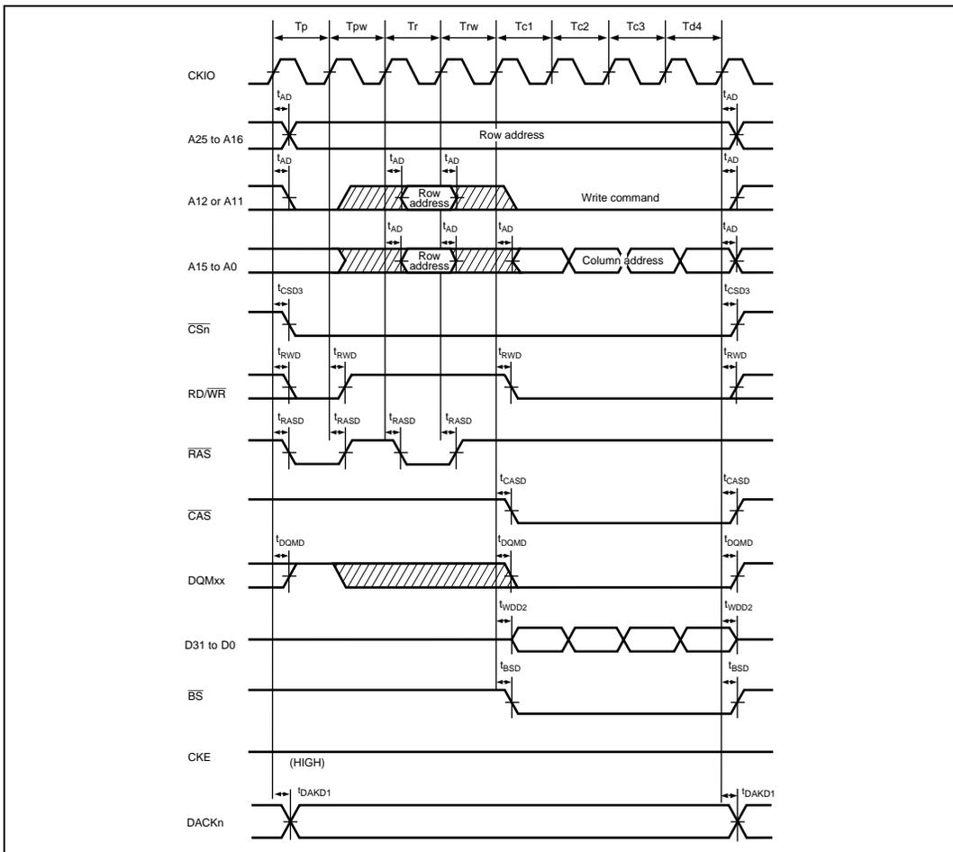
**Figure 24.36 Synchronous DRAM Burst Write Bus Cycle
