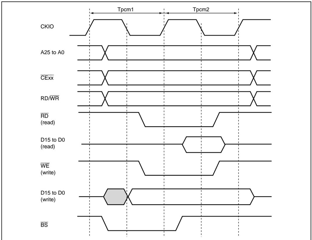
**Figure 8.32 Basic Timing for PCMCIA Memory Card Interface**
