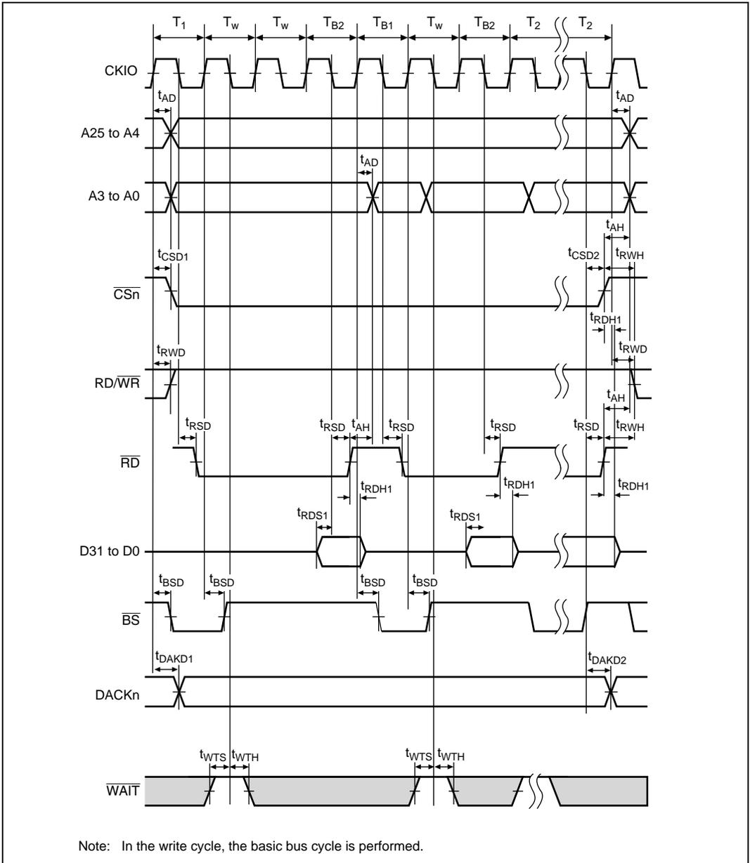
**Figure 24.20 Burst ROM Bus Cycle (Two Waits)**
