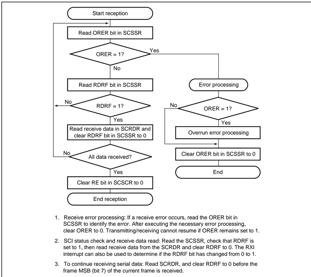
**Figure 14.21 Sample Flowchart for Serial Data Receiving**
