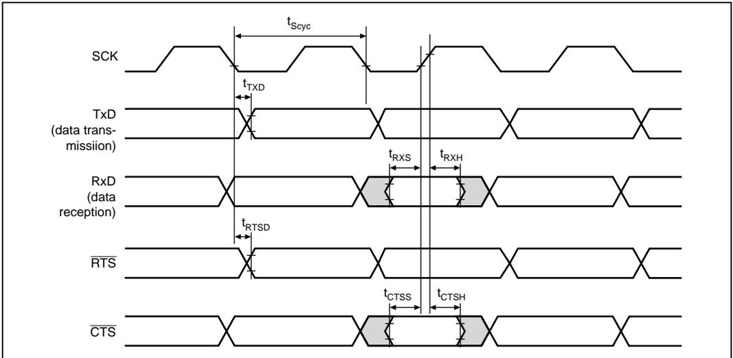
**Figure 24.51 SCI I/O Timing in Clock Synchronous Mode**
