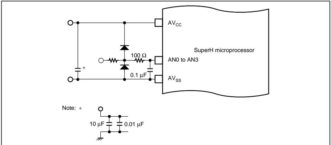
**Figure 19.11 Example of Analog Input Protection Circuit**
