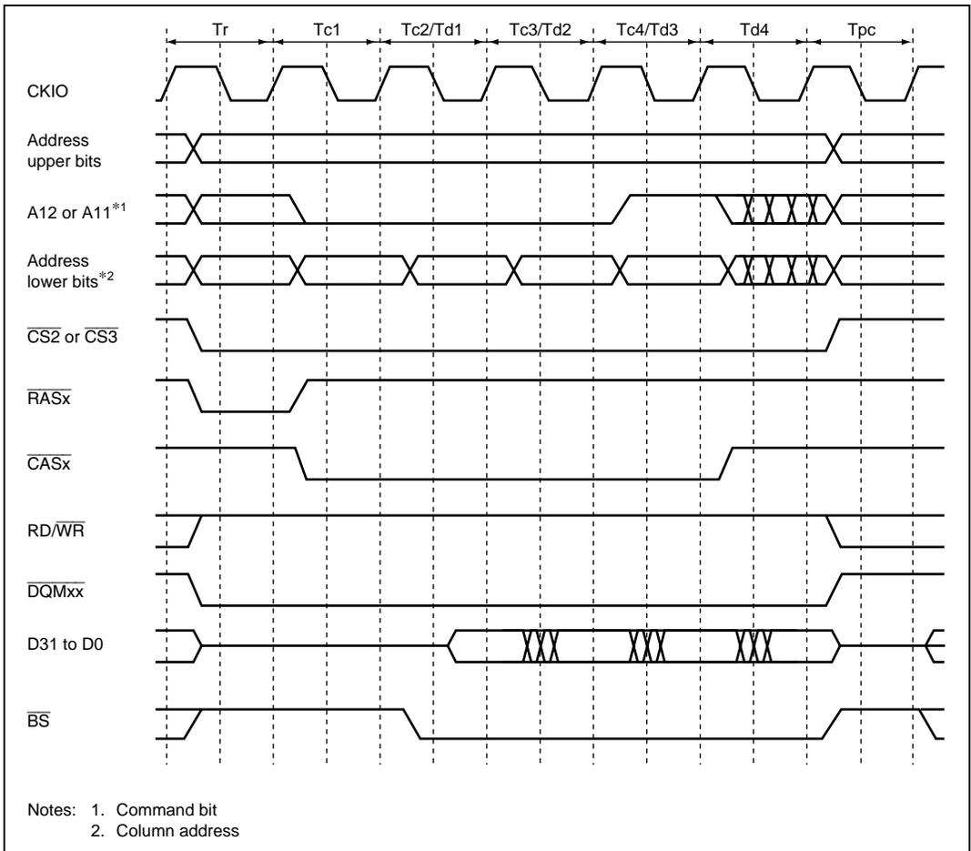
**Figure 8.13 Basic Timing for Synchronous DRAM Burst Read**
