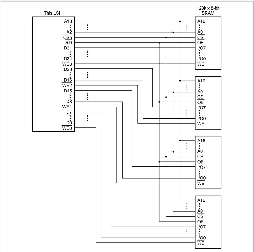
**Figure 8.6 Example of 32-Bit Data-Width Static RAM Connection**
