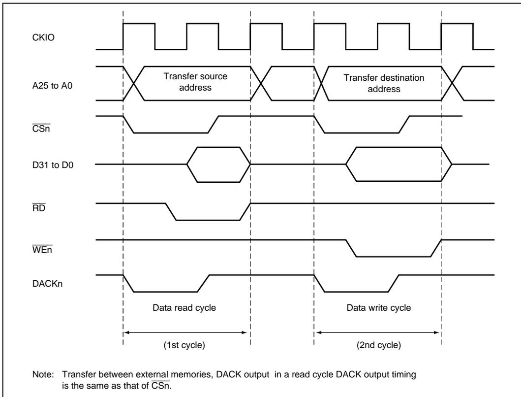
**Figure 9.6 Example of DMA Transfer Timing in the Direct Address Mode
