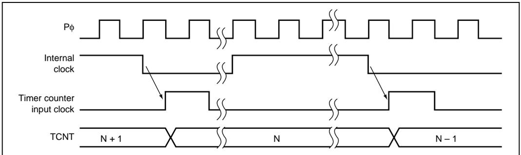
**Figure 12.4 Count Timing when Internal Clock Is Operating**
