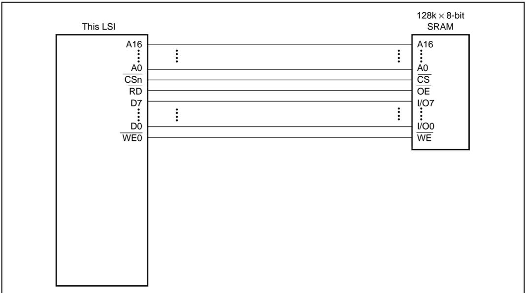
**Figure 8.8 Example of 8-Bit Data-Width Static RAM Connection**
