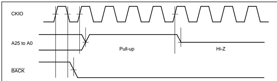
**Figure 8.40 Pins A25 to A0 Pull-Up Timing**
