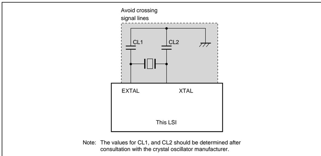
**Figure 10.2 Points for Attention when Using Crystal Oscillator**
