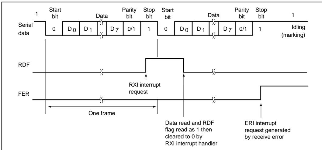
**Figure 16.11 Example of SCIF Receive Operation
