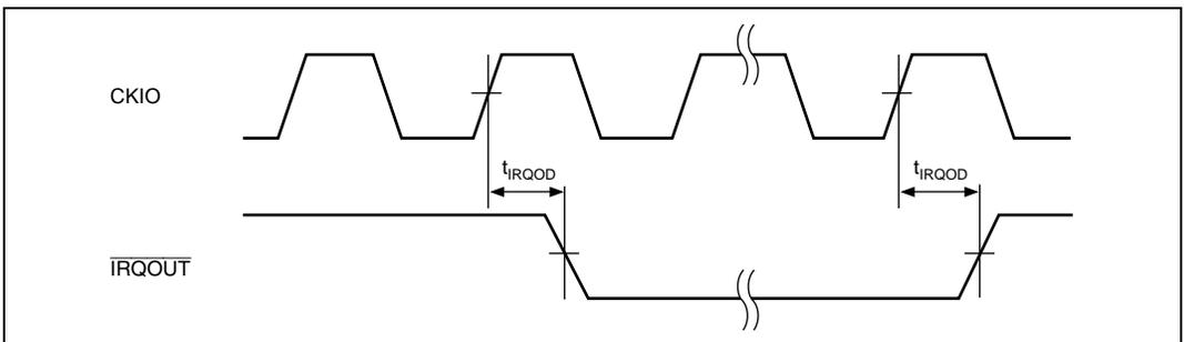
Figure 24.13  $\overline{\text{IRQOUT}}$  Timing
