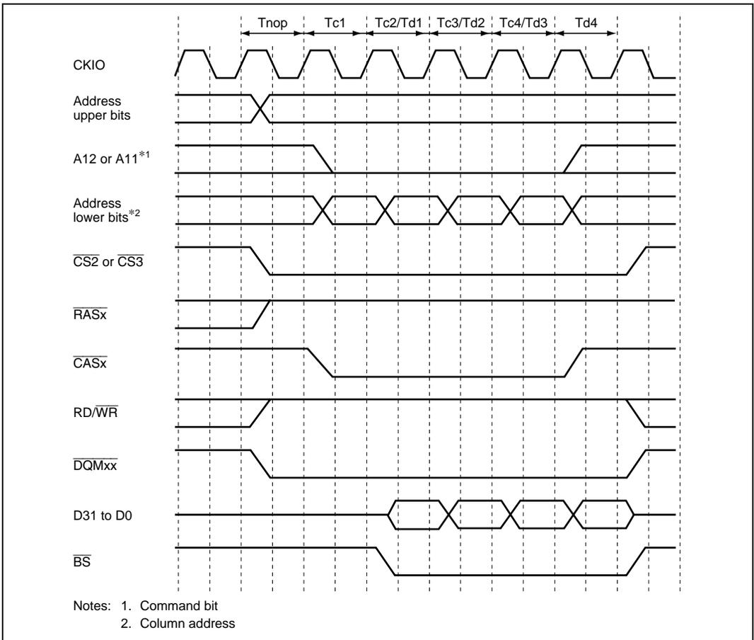
**Figure 8.19 Burst Read Timing (Same Row Address)**
