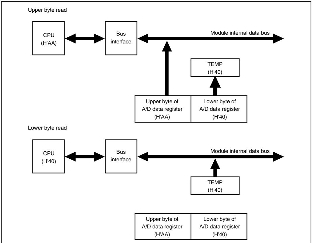
**Figure 19.2 A/D Data Register Access Operation (Reading H'AA40)**
