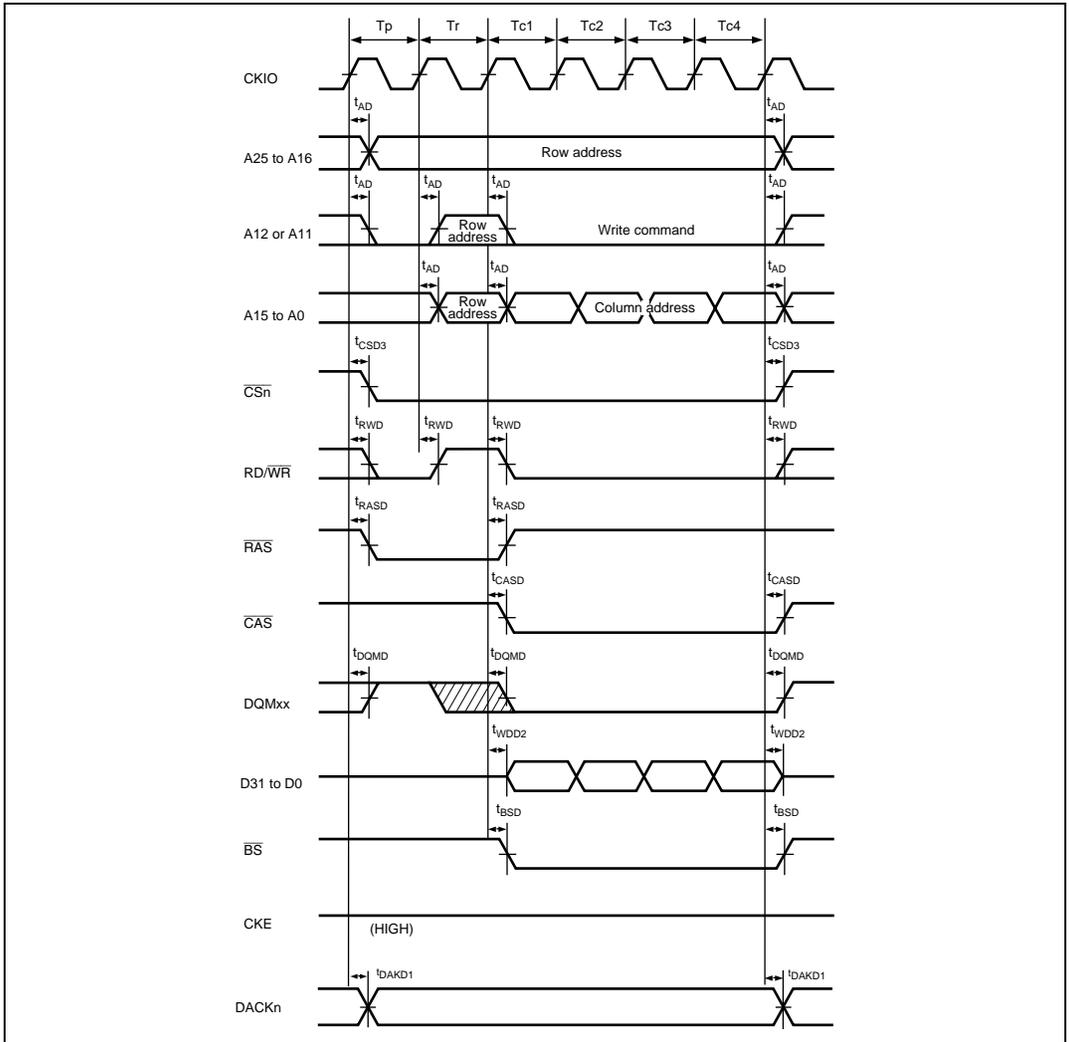
**Figure 24.35 Synchronous DRAM Burst Write Bus Cycle
