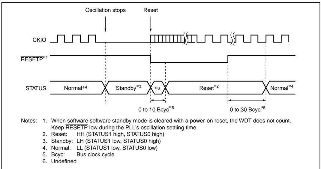
**Figure 22.5 Software Standby to Power-On Reset STATUS Output**
