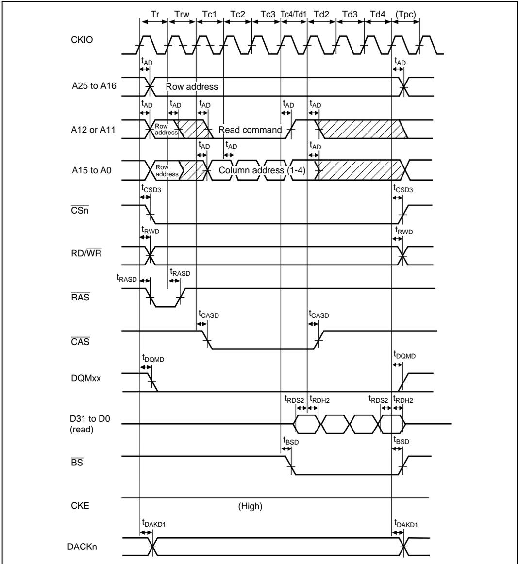
**Figure 24.25 Synchronous DRAM Read Bus Cycle
