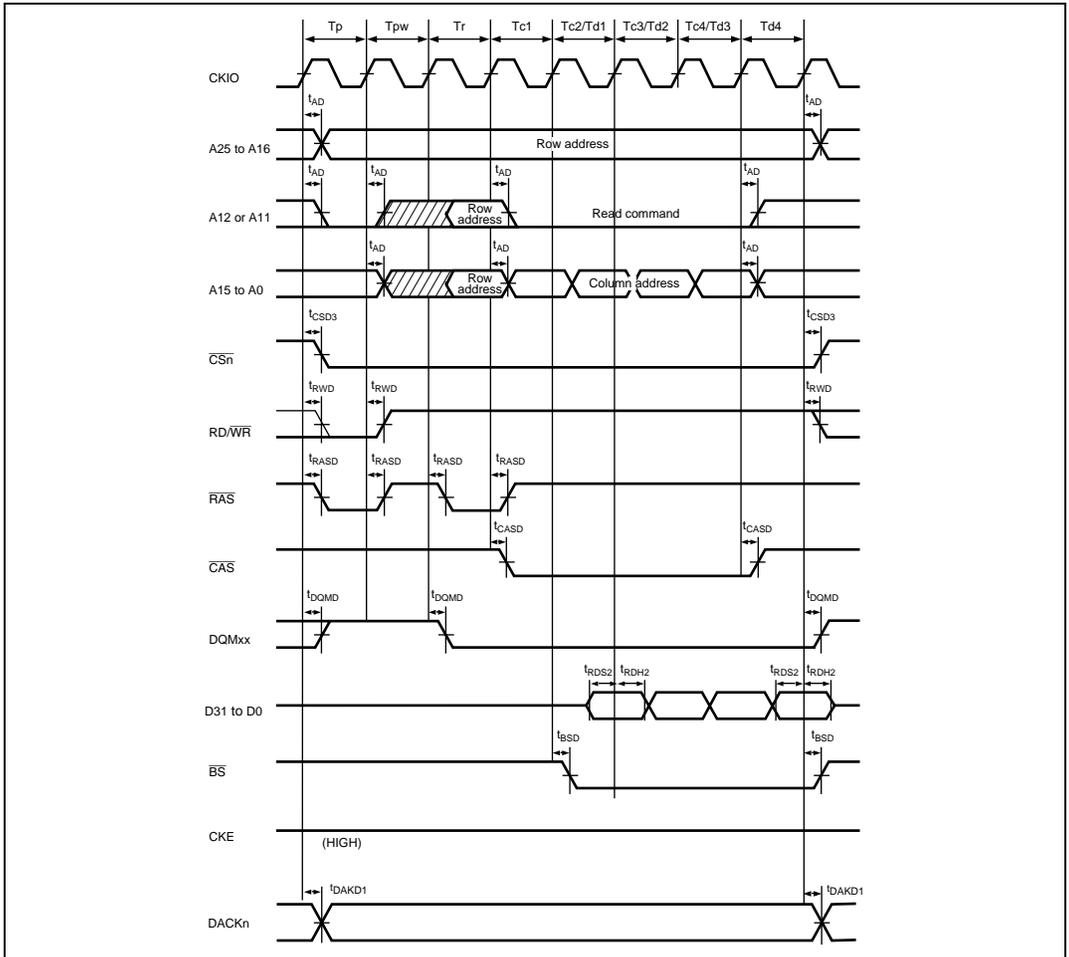
**Figure 24.33 Synchronous DRAM Burst Read Bus Cycle**
