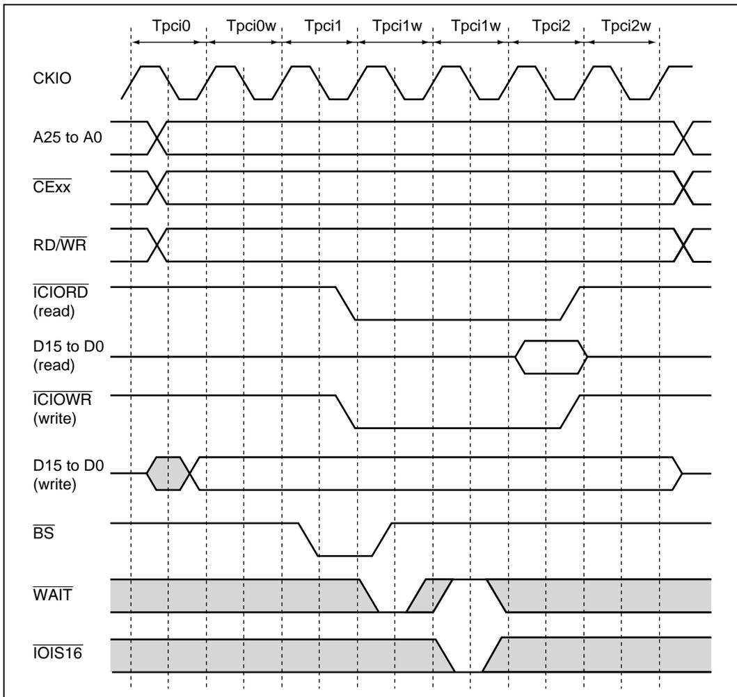
Figure 8.37 Wait Timing for PCMCIA I/O Card Interface
