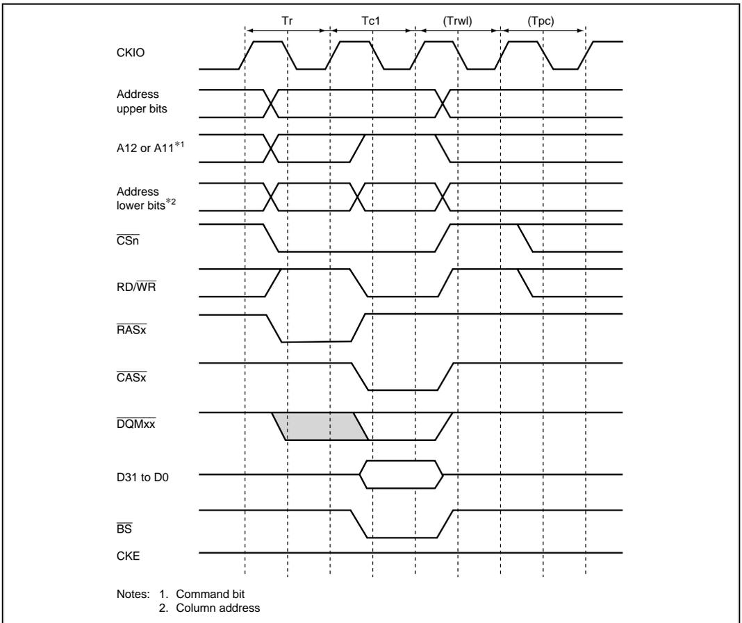
**Figure 8.17 Basic Timing for Synchronous DRAM Single Write**
