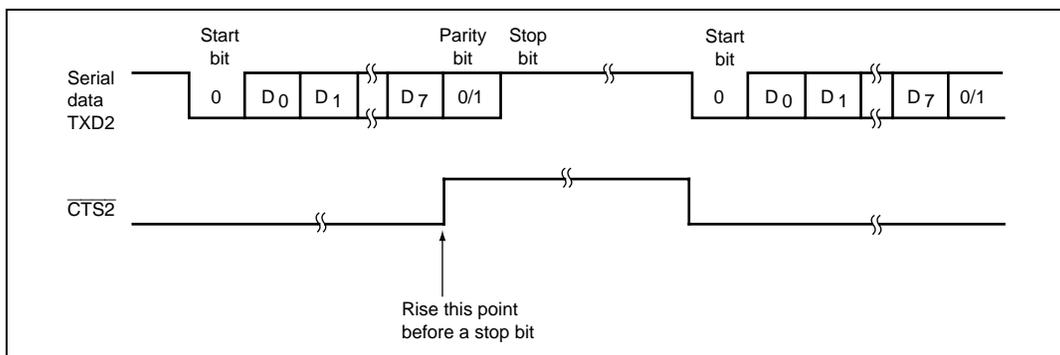
**Figure 16.8 Example of Operation Using Modem Control ( $\overline{\text{CTS2}}$ )**
