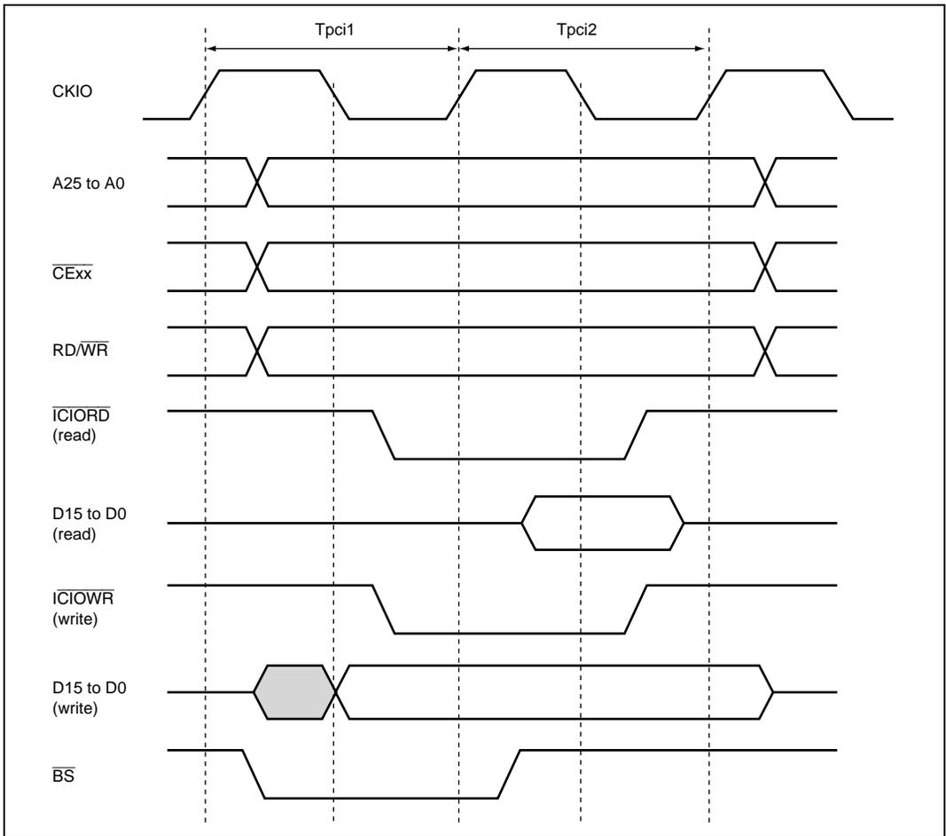
**Figure 8.36 Basic Timing for PCMCIA I/O Card Interface**
