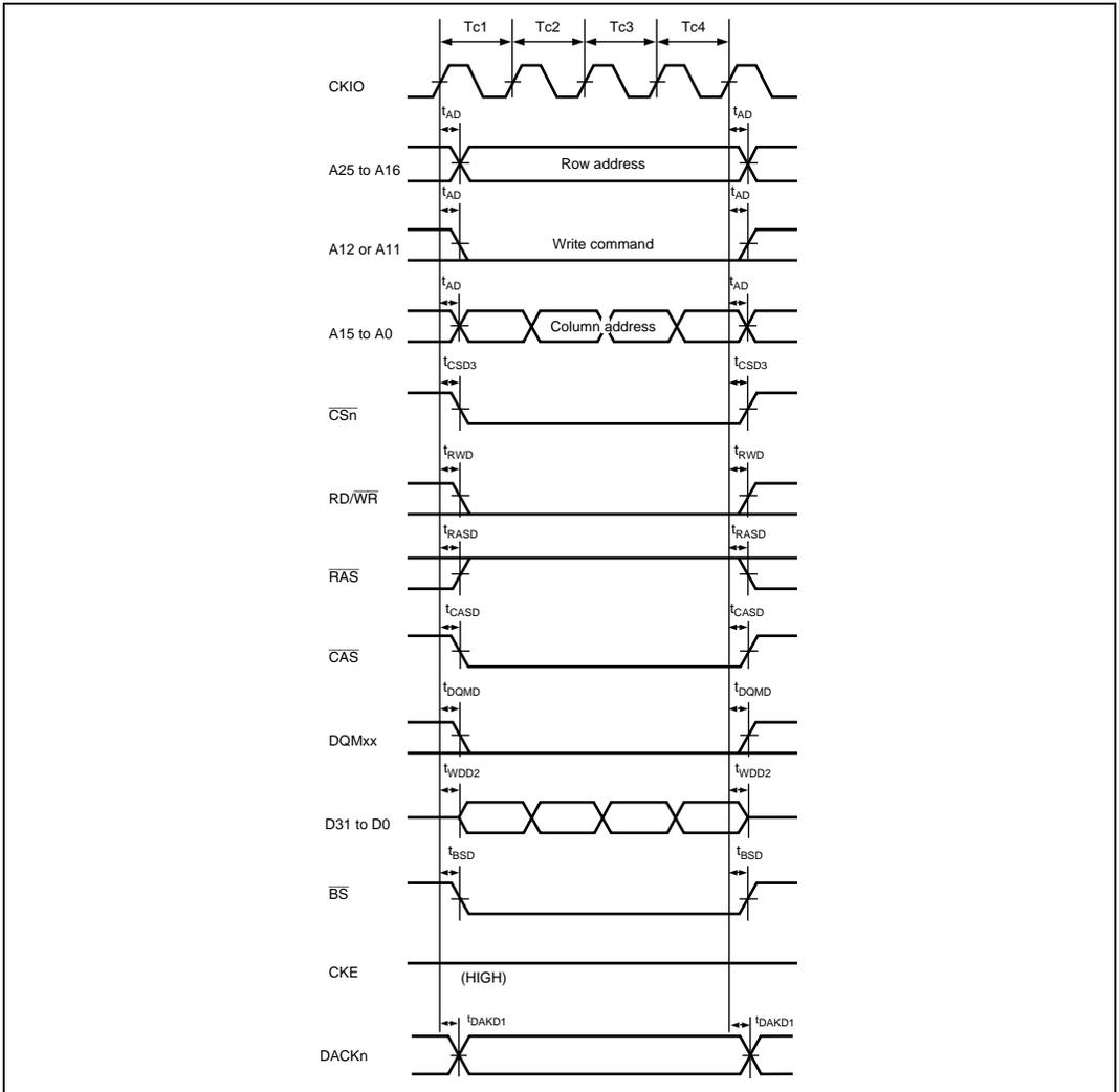
**Figure 24.34 Synchronous DRAM Burst Write Bus Cycle
