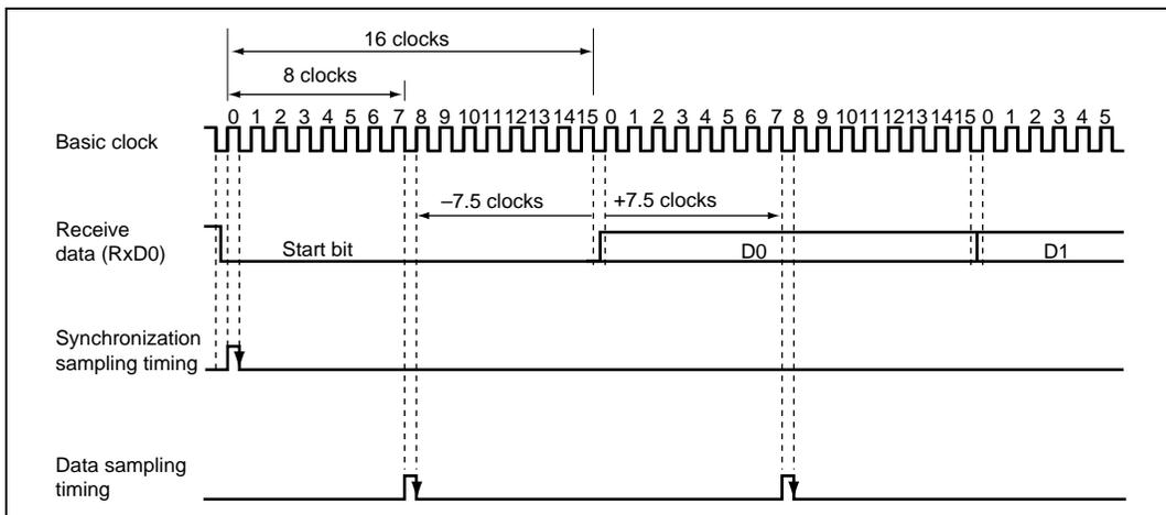
Figure 14.24 Receive Data Sampling Timing in Asynchronous Mode
