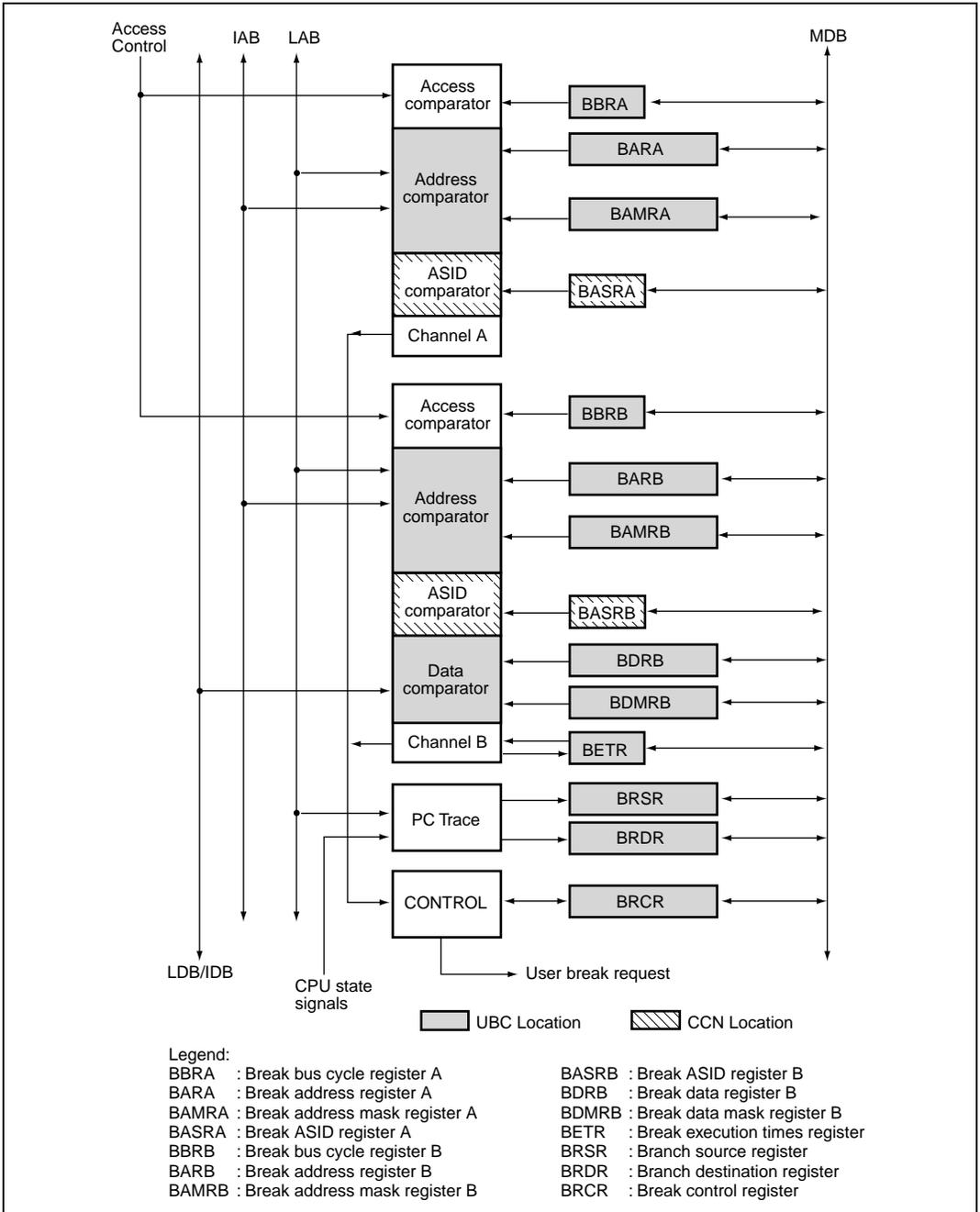
**Figure 7.1 Block Diagram of User Break Controller**
