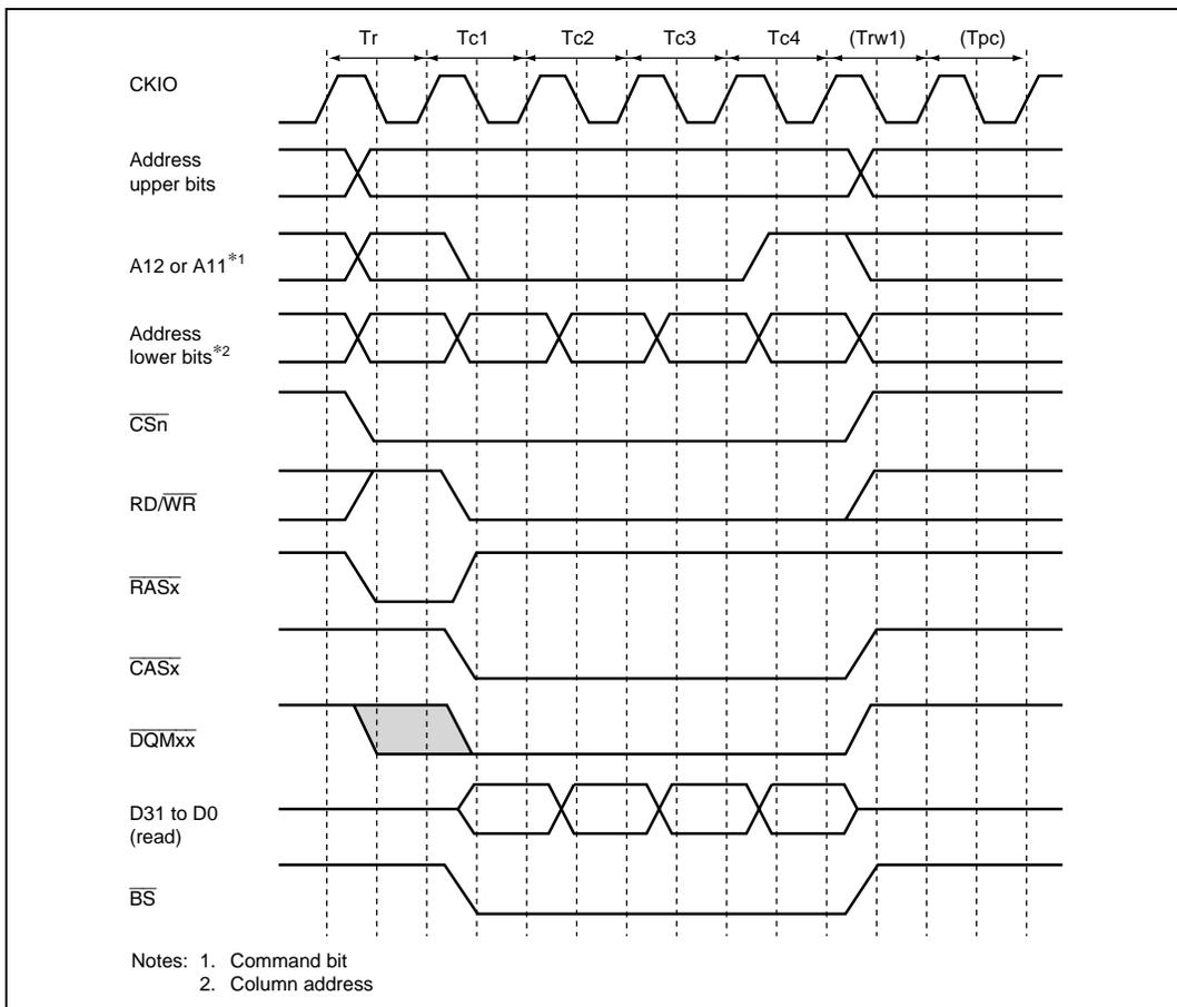
**Figure 8.16 Basic Timing for Synchronous DRAM Burst Write**
