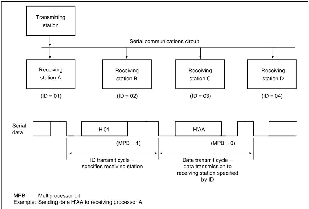
**Figure 14.12 Communication Among Processors Using Multiprocessor Format**
