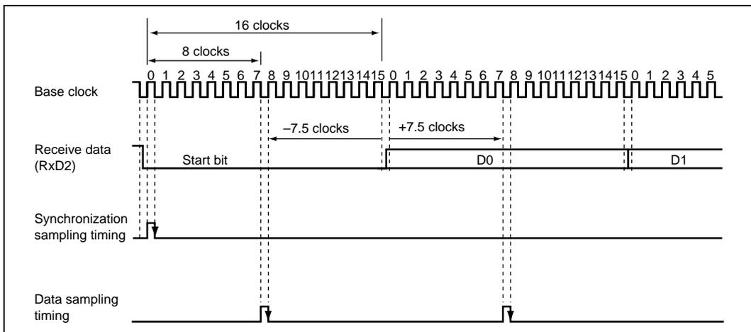
**Figure 16.13 Receive Data Sampling Timing in Asynchronous Mode**
