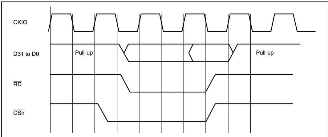
**Figure 8.41 Pins D31 to D0 Pull-Up Timing (Read Cycle)**
