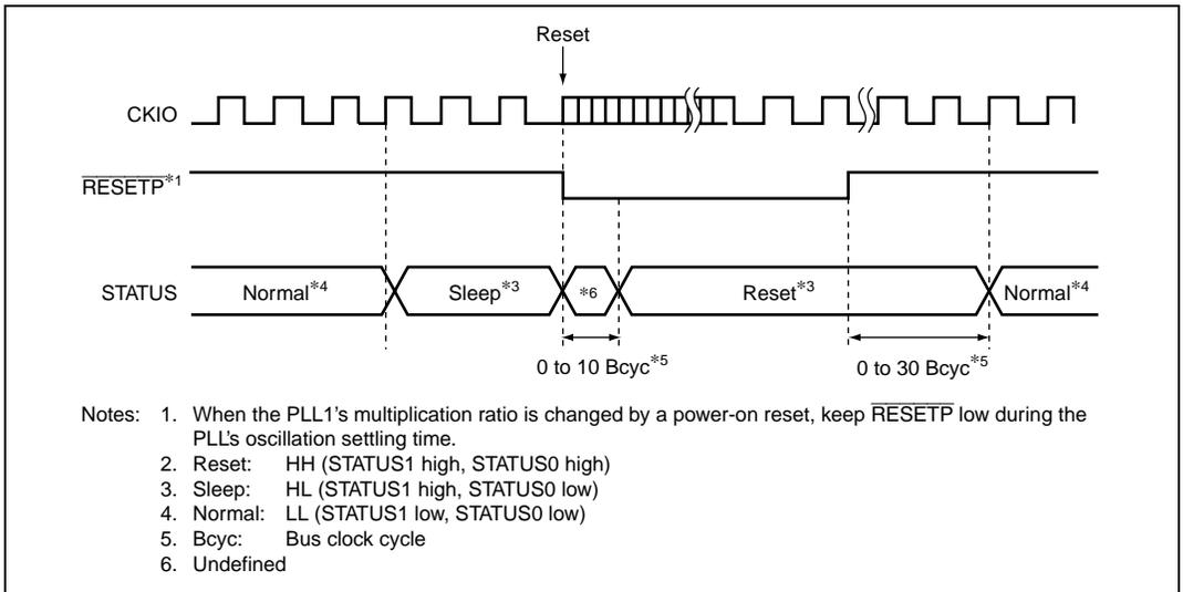
Figure 22.8 Sleep to Power-On Reset STATUS Output
