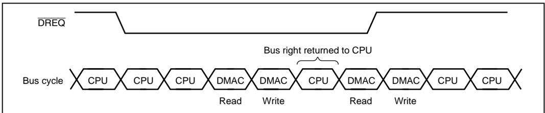
**Figure 9.14 DMA Transfer Example in the Cycle-Steal Mode**
