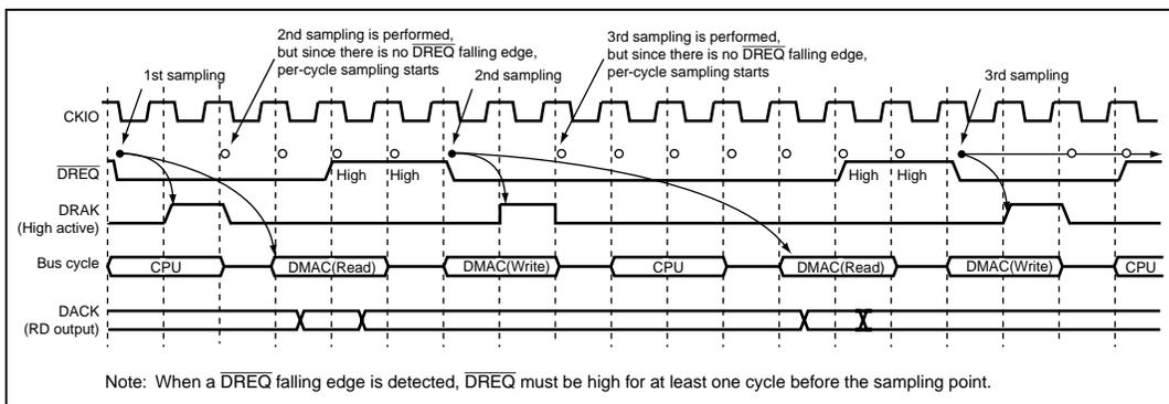
**Figure 9.21 Cycle-Steal Mode, Edge input (CPU Access: 2 Cycles)**
