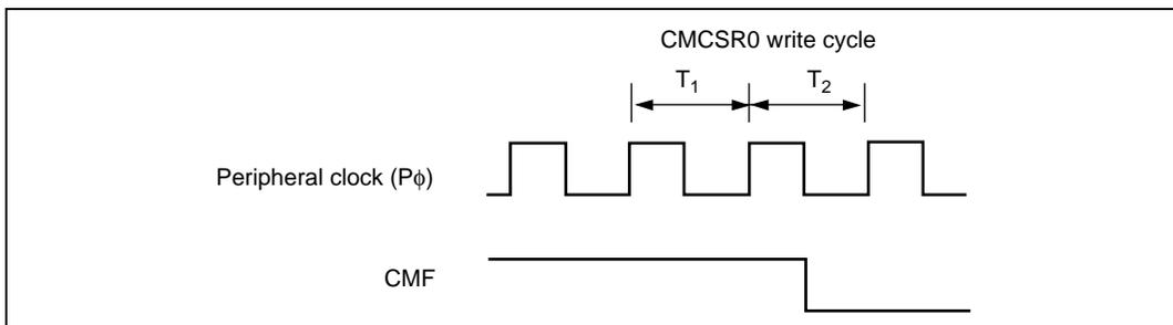
**Figure 9.30 Timing of CMF Clear by the CPU**
