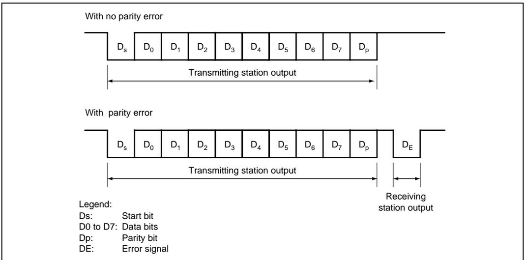
**Figure 15.3 Data Format for Smart Card Interface**
