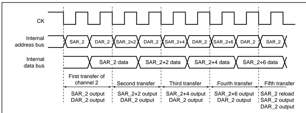
**Figure 9.25 Timing Chart of Source Address Reload Function**
