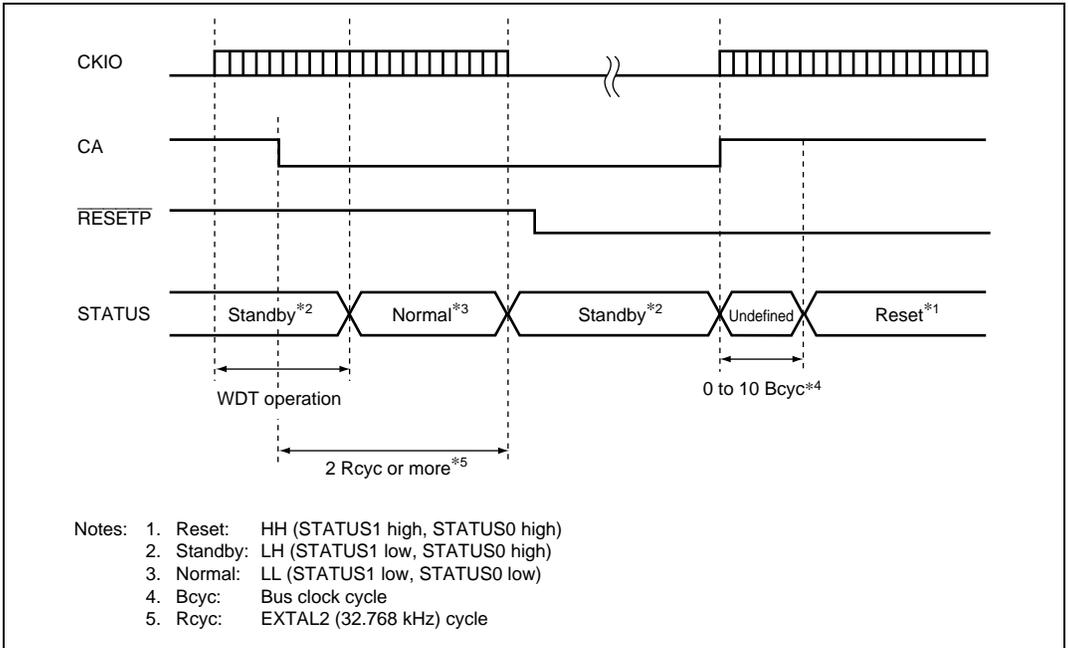
**Figure 22.11 Hardware Standby Mode Timing**
