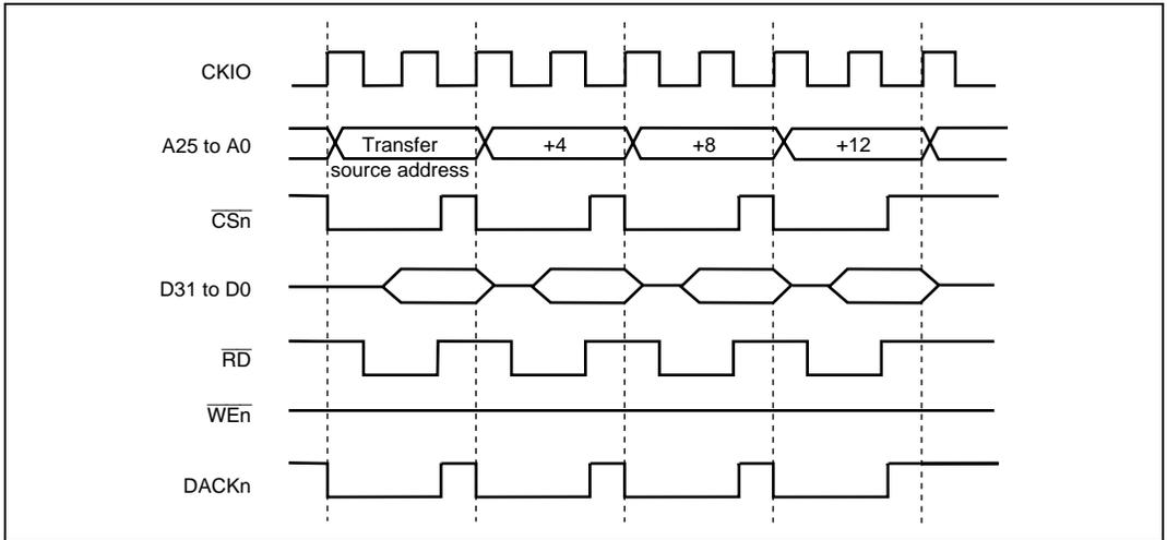
**Figure 9.13 Example of DMA Transfer Timing in the Single Address Mode**
