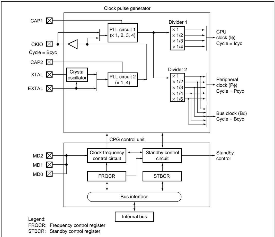
**Figure 10.1 Block Diagram of Clock Pulse Generator**
