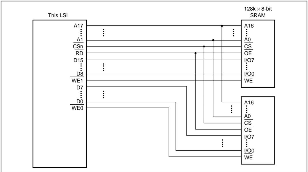
**Figure 8.7 Example of 16-Bit Data-Width Static RAM Connection**
