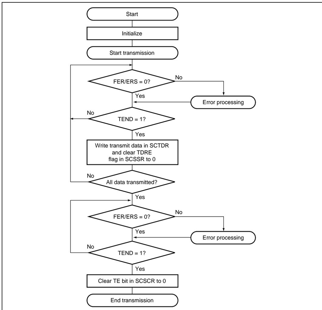
**Figure 15.6 Transmission Flowchart**
