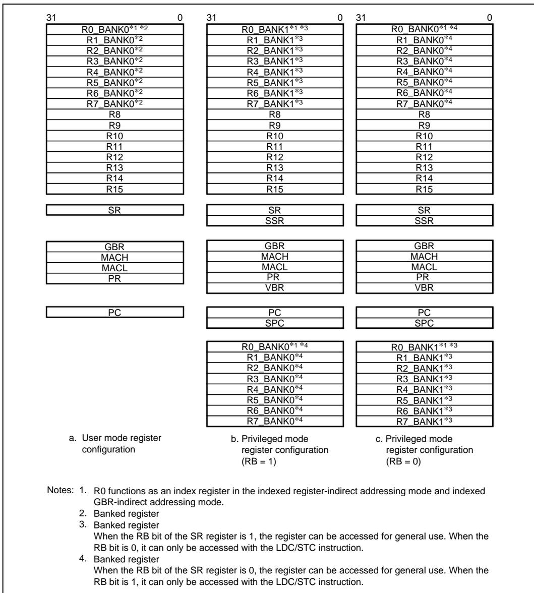
**Figure 2.1 Register Configuration**
