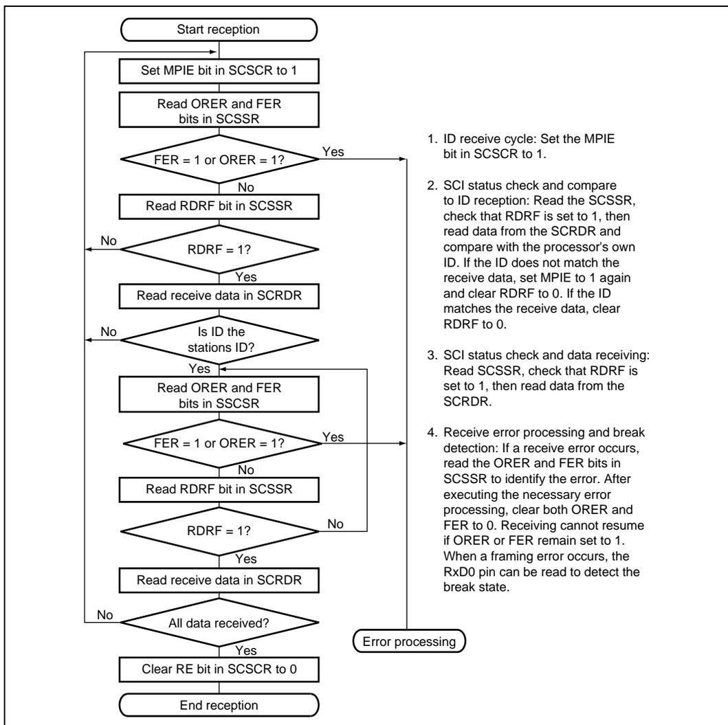
**Figure 14.15 Sample Flowchart for Receiving Multiprocessor Serial Data**
