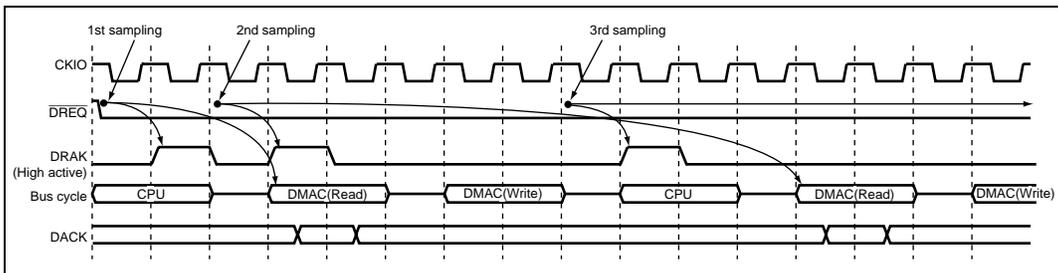
**Figure 9.17 Cycle-Steal Mode, Level Input (CPU Access: 2 Cycles)**
