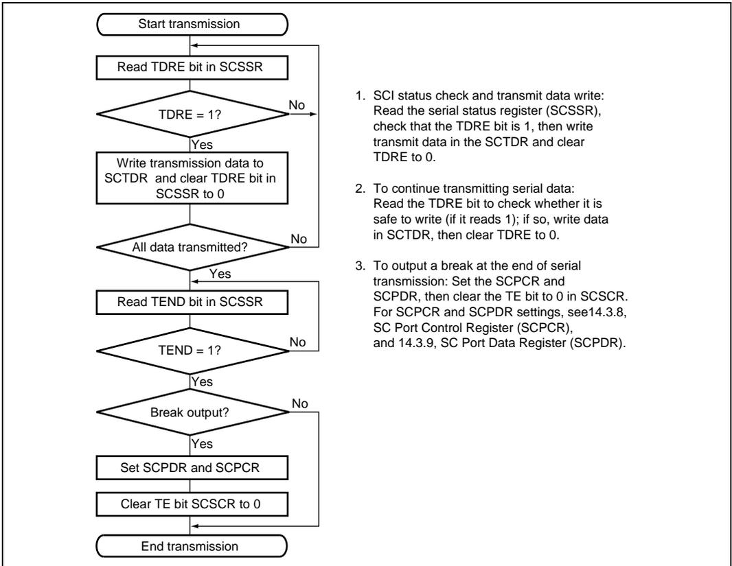
**Figure 14.8 Sample Flowchart for Transmitting Serial Data**
