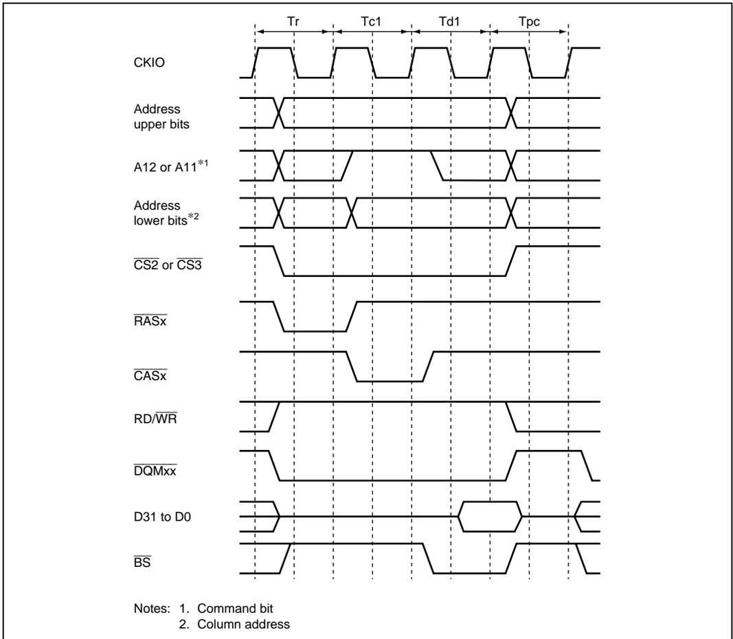
**Figure 8.15 Basic Timing for Synchronous DRAM Single Read**
