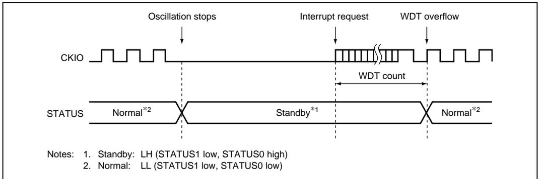
**Figure 22.4 Software Standby to Interrupt STATUS Output**
